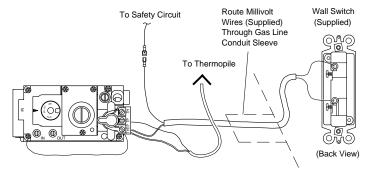
*Note*: If any of the original wire as supplied must be replaced, use 18 AWG TYPE CL2 (UL) 105 C (25 ft. length MAXIMUM) or equivalent.
